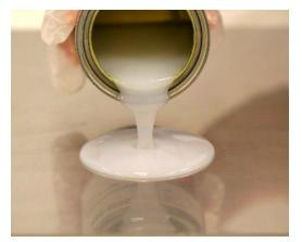
MED-6655 one-part, 100mol% fluorosilicone adhesive/sealant dispersed in Tert-Butyl Acetate.
